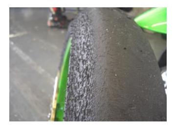
If your tire is showing bad wear patterns on the edge third, where the start of the wear pattern (the bit closest to the middle of the tire) follows the circumference of the tire uniformly, you can be pretty sure you're suffering from geometry tear and have too much weight on the front.
