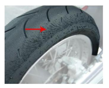
At first glance it's quite similar to cold tear but because the whole tire is overheating instead of just the surface, the rubber comes off with less effort as opposed to being ripped off a cold carcass like you see with cold tear, this then means hot tearing isn't as deep.
