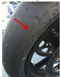
where they gain significant heat, when they cool down again (this is one heat cycle) the oils in the tire will often come to the surface. When you go back out and ride the bike these surface oils are scrubbed off and it's only when you come back in and let the tires cool down again that you'll see more oils coming to the surface.
