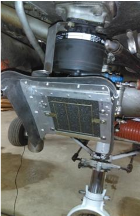
New air intake; the original was melted due to an engine fire on start-up years ago. Above the air box is a new vacuum pump to drive the gyro instruments.
